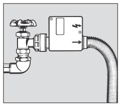
The water inlet hose comes equipped with a 3/4" female hose thread connector. This can be directly connected to a shut off valve with 3/4" male hose thread ends.
